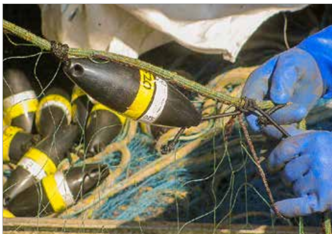
Figure 3: PALfi attached to gillnet floatline.
