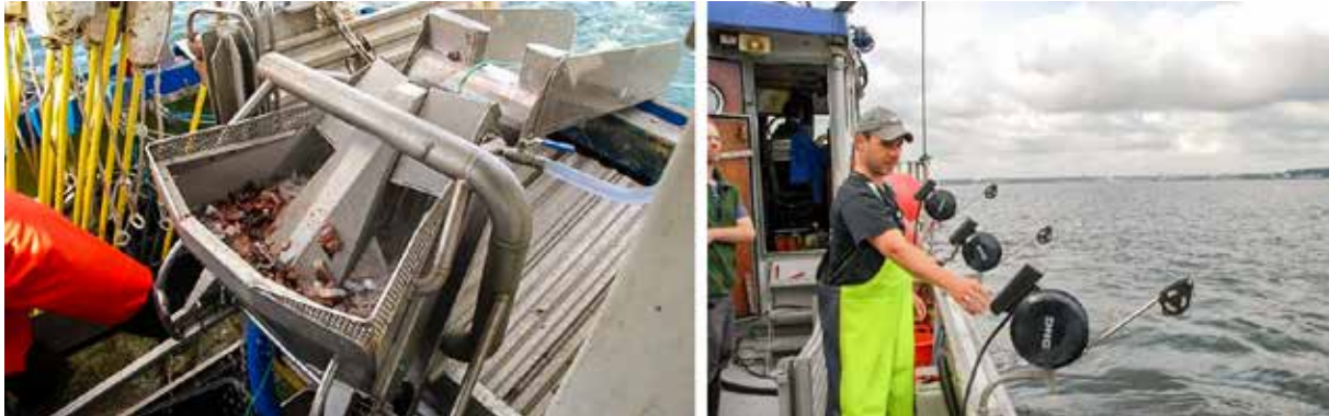
Figure 2 and 3: Alternative fishing gear in field studies : Oilwind longline system (baiter) and DNG jigging machines (NABU/K.Detloff).
