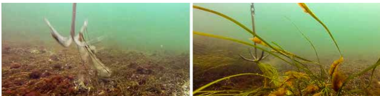
Figure 6: Impacts are to a large degree eliminated if hauling is carried out with the vessel positioned directly above the anchor. Anchor prongs point upwards and removal of algae and disturbance to sediments is usually avoided.
