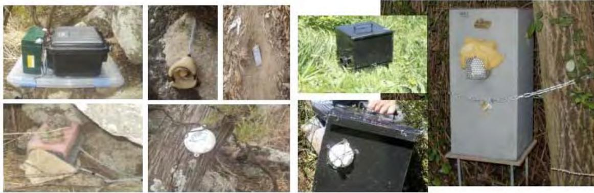
**Figure 4:** Examples of location and protection of recording systems.
