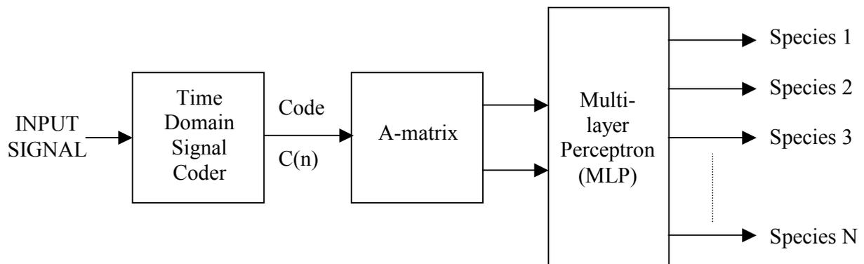
**Figure 4:** Schematic diagram of the Intelligent Bioacoustic Identification System (IBIS).
