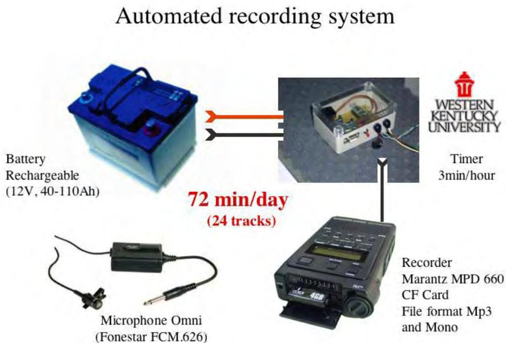
**Figure 3:** Diagram of the automated recording system.
