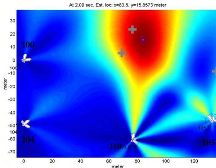
**Figure 2:** Results of the collaborative localization algorithm, presented as a 2D pseudo-likelihood map. One can see that the individual estimations of the angle of arrival (AOA) for each node (black lobes represent the likelihood for source AOA) are combined using their location as estimated by the self-calibration process.
