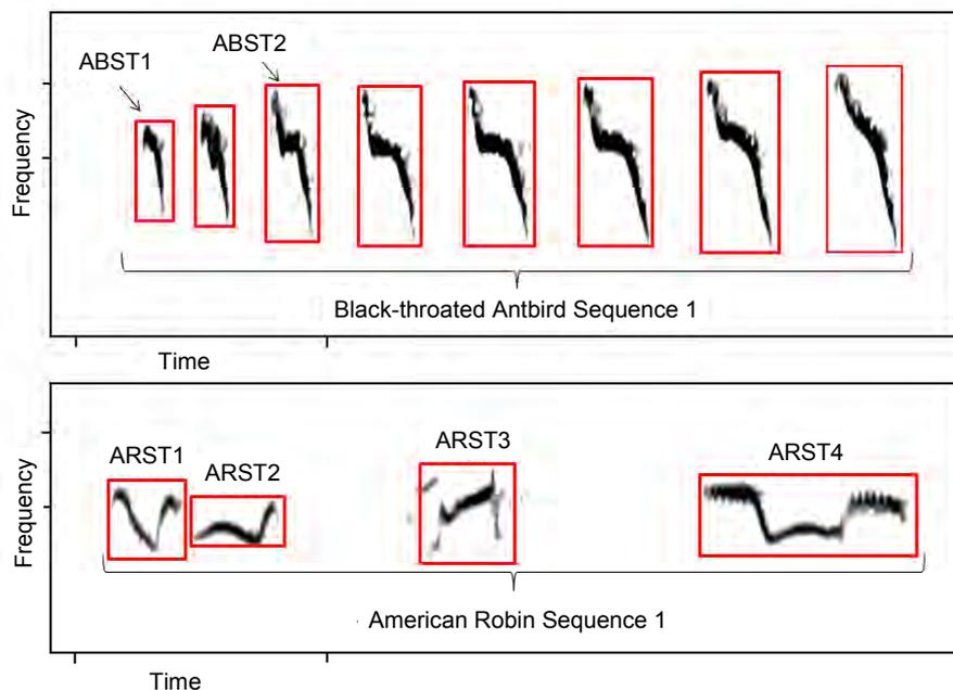
**Figure 3:** Sequence recognition with composite HMMs. The individual calls are found with the first layer HMM, and the sequence of these calls is classified with the second layer HMM.
