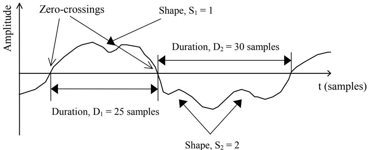
**Figure 3:** Time Domain Signal Coding of a Waveform.
