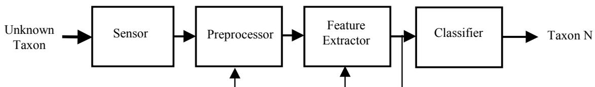
**Figure 1:** Schematic diagram of a typical automated taxon identification system.
