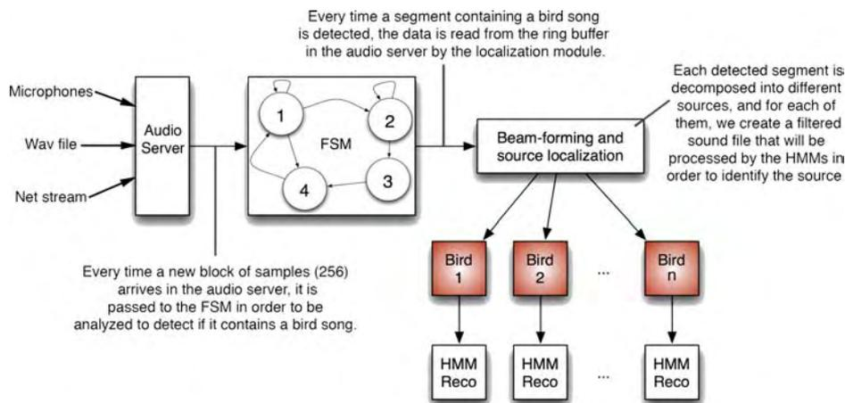
**Figure 1:** The workflow of the whole architecture developed during this project. The Audio Server task is to store all the incoming audio data (the data source is chosen when the server is started) into an indexed ring buffer. Then the incoming signals are processed to detect eventual bird songs. Every time a song is detected, it will be localized and beamformed, and each resulting sound file will be processed with HMM to recognize the species, and finally stored along with other metadata.
