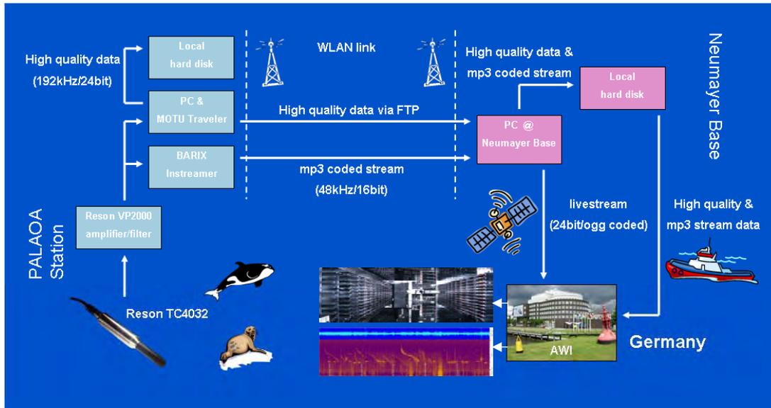
**Figure 8:** Audio data streams, from the water to long term archival and web broadcasting
